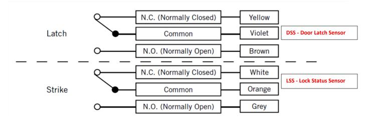
The wiring diagram is shown for the lock being locked, and door closed.
