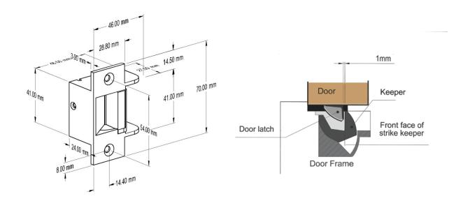
As drawn in the diagram, there should be a 1mm gap between the door latch and the front face of the strike keeper, preventing the door from creating back pressure on the strike keeper when the door is closed.
