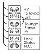
Wiring using bolt sensing. Solenoid will only power when the door is closed (PTL fail safe only) PDFS0012 June 2023
