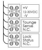
Standard wiring. Contacts are N.C. with door closed and secure.
