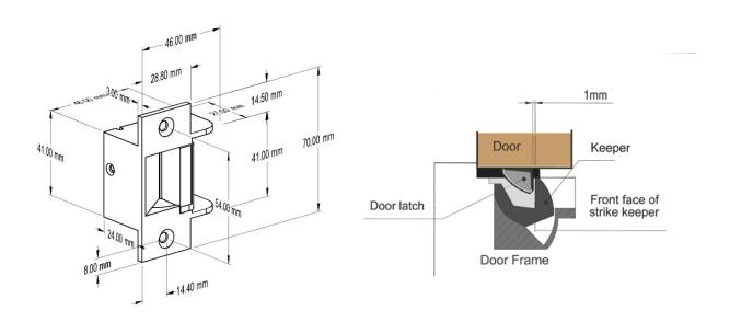
As drawn in the diagram, there should be a 1mm gap between the door latch and the front face of the strike keeper, preventing the door from creating back pressure on the strike keeper when the door is closed.
